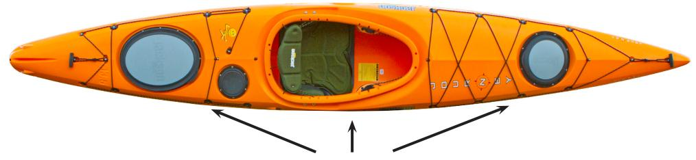
Drain hatches, cockpit, and gear such as sponges and pumps
